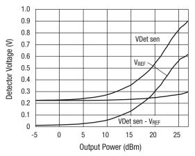
Built-In Detector Responses at V<sub>CC</sub>Det = 2.5 V
